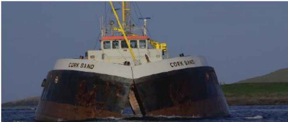
Figure 3-3: Split Barge in Operation
