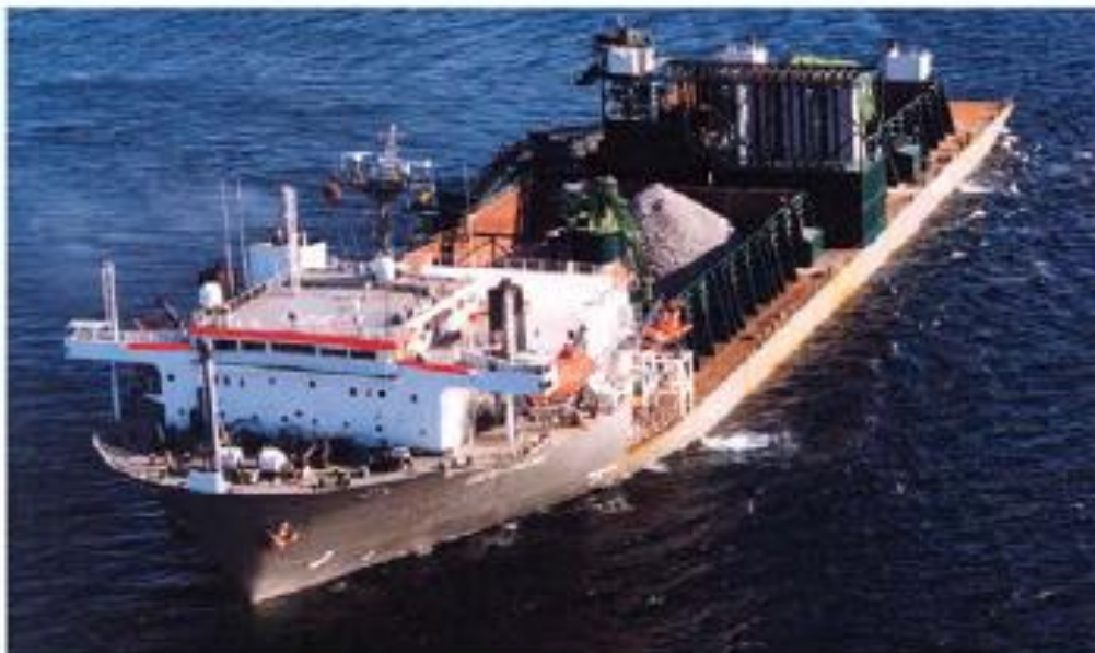
Figure 3-4: Fallpipe Vessel – Rockpiper
